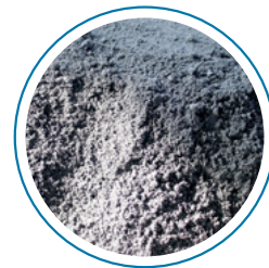
Iron silicate fines, similar to mineral flour
